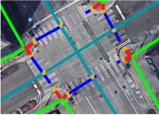
Figure 11 An intersection fully-mapped for crossings, curbs, sidewalks, and links.
